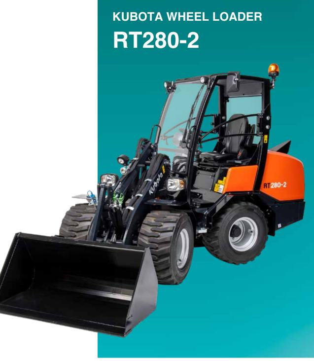
Engine output (PS): 50 Machine weight (kg): 2600 / 2750
