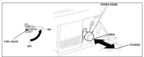
Turn the fuel valve to the ON position. To start a cold engine, pull the choke knob out to the CLOSED position. To restart a warm engine, leave the choke knob in the OPEN position.
