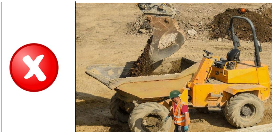
Figure 10 – Example of an operator within the loading activity danger area
