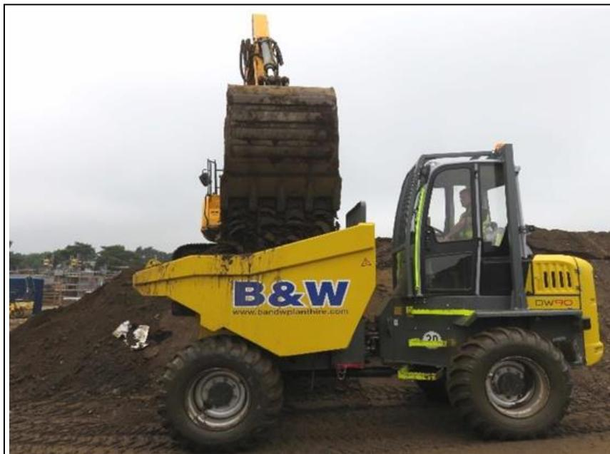
**Figure 14 – Example of Side Loading Using the Prescribed Method**
