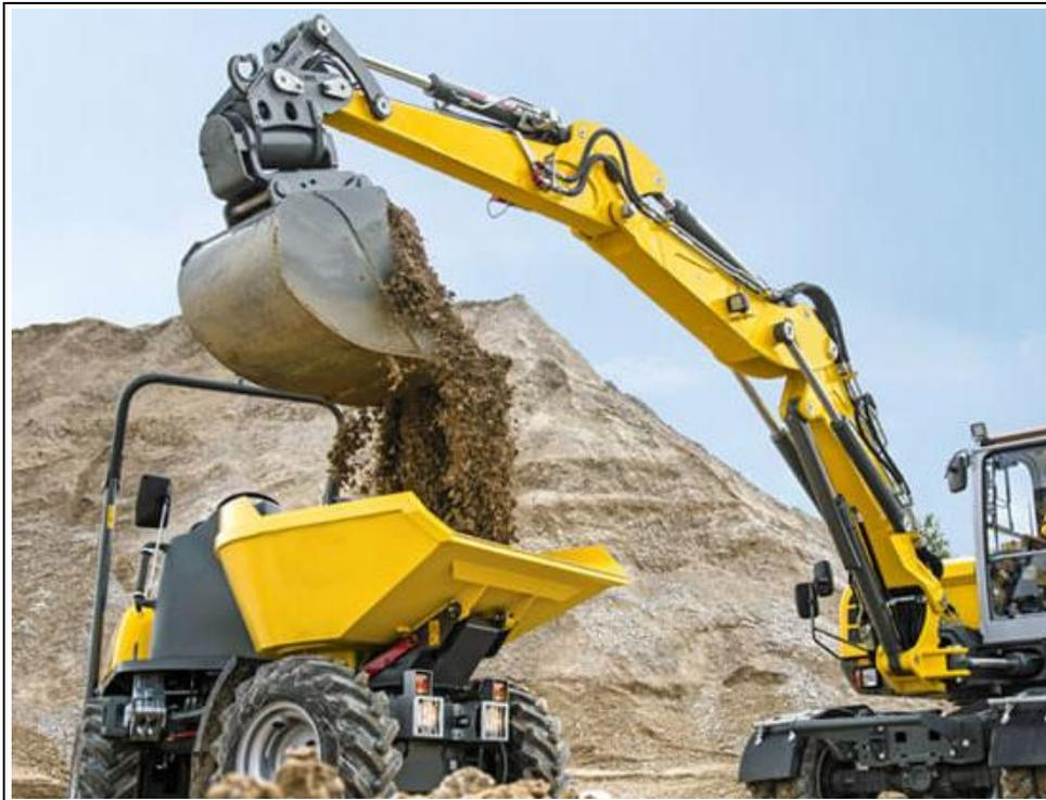
**Figure 16 – Example of potential overloading**
