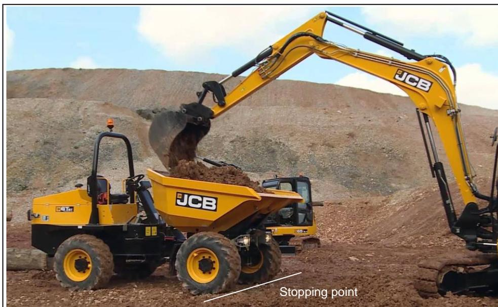
**Figure 13 – Example of Forward Loading**
