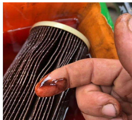
Blocked Fuel Filter
