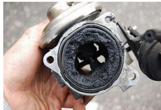
Blocked Exhaust Gas Recirculation Valve
